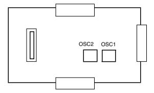
OSC1 ...Oscillator (42.3158MHz): For 400dpi Printer OSC2 ...Oscillator (95.2106MHz): For 600dpi Printer
